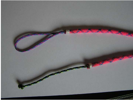
Pic 5: Splice a loop in the one end of the sheet (use a 3mm coreless strap) and a piece of 3mm Dyneema in the other end. Tie a stopper knot in the strap.
