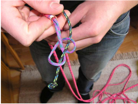
Pic 6: Bring the two ends together as shown in the picture (the coreless loop will wedge around the Dyneema strap and guarantees a strong assembly)
